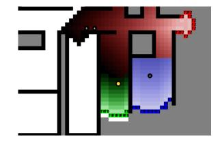
Fig. 7. Illustration . Wavefronts are stopped on the encounter of the yellow robot computing its assignment. Color code : white=explored, gray=unknown, black=walls, red-green-blue=frontier and gradient wavefront propagation result, only the wavefront closest to the frontier is shown where waves are superimposed.
