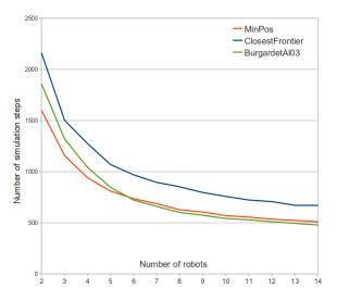
Fig. 6. Results from the exploration of the hospital environment when varying the number of robots
