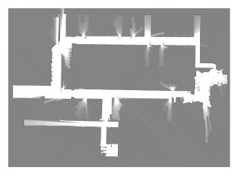
Fig. 3. Illustration of a map (63m long building) created without loop closure.
