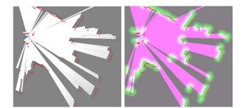
Fig. 2. New scan located in the map (Left) and surimposed maps: occupancy, distances and new scan (Right)
