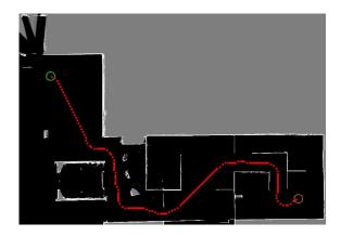
Fig. 8. Exemple of a planned trajectory keeping away from obstacles
