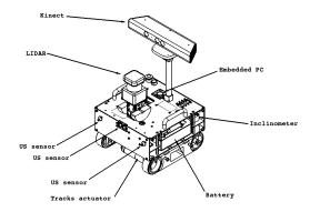
Fig. 9. Specifications of the MiniRex robot.
